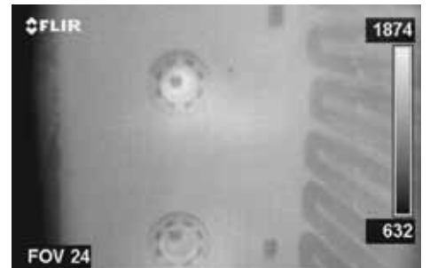
Due to the built in flame filter the FLIR GF309 thermal imaging camera can see through flames and even measures the temperatures behind the flames.
